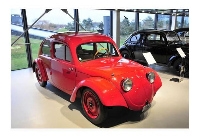
the second prototype of the **Beetle** (known at that time as the **KdF-Wagen** ) in 1935 was the first design with definitive features of the future **Beetle**
