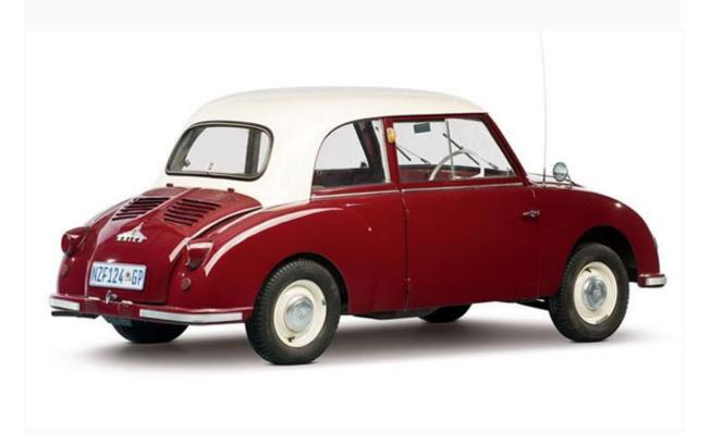
The **Maico 500** was a 4-seat version of the **Champion 400** and had a larger 452cc engine; It was distinguished from the older versions by its larger size and its rectangular roof, and it would be the model on which the **Alcre Susana would be based**.
